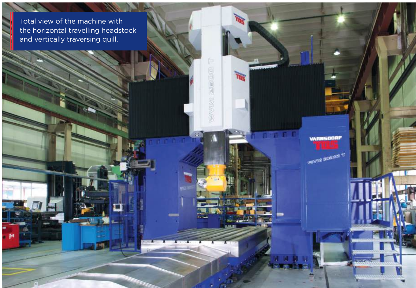
View of the orthogonal 2 axis automatically indexed milling head.
