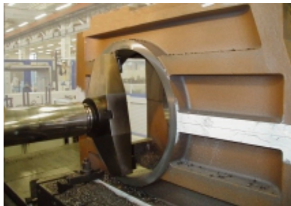
MILLING AND DEEP DRILLING INTO THE PUMP BODY
