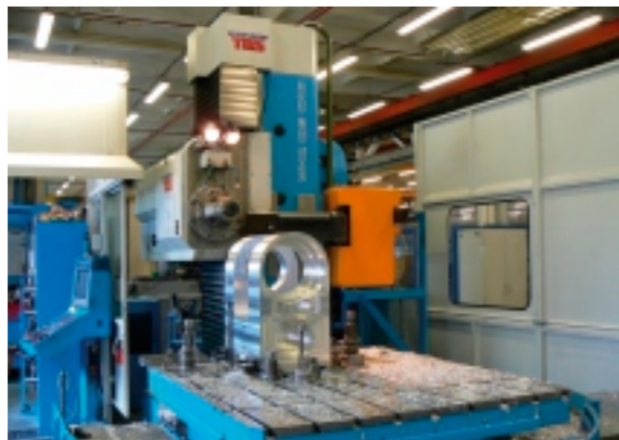
MILLING OF A MILLING HEAD ALUMINIUM BODY
