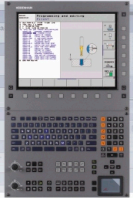
CONTROL PANEL OF HEIDENHAIN iTNC 530 CONTROL SYSTEM
