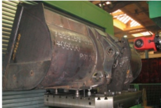
MILLING OF A VALVE
