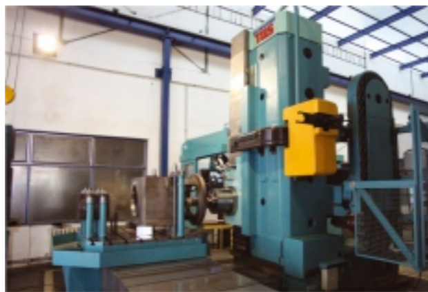
MILLING OF A VALVE
