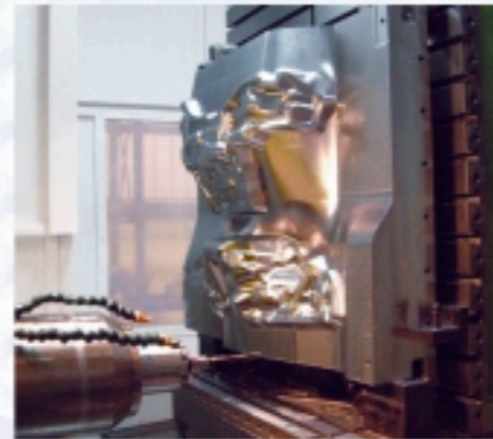
MILLING OF AN INJECTION MOULD
