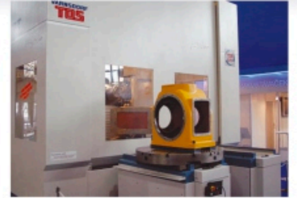
MILLING AND DRILLING OF A COMPRESSOR BODY
