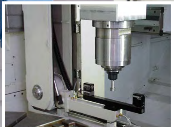
ROTATING TOOL : PRESETTING
