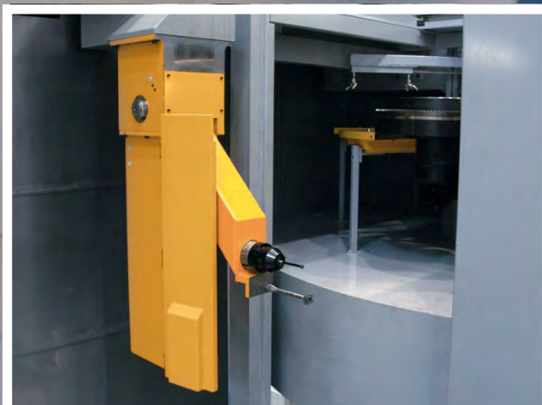
TURNING TOOL : PRESETTING
