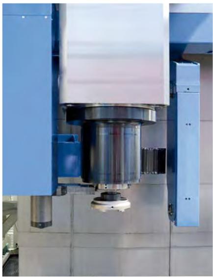
VERTICAL MILLING HEAD
