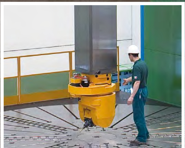
UNIVERSAL HEAD 2 CONTINUOUS AXES
