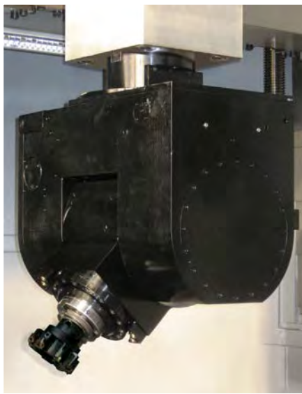
UNIVERSAL POSITIONING HEAD
