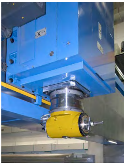
HORIZONTAL MILLING HEAD
