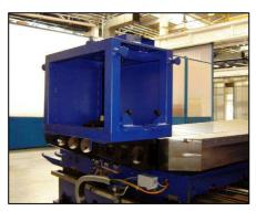
The support improves significantly the putting off the optional accessories determined for the automatic control of the PICK UP change. Its execution (number of storage places, covers, etc.) is subject to prior consultation with the manufacturer.
