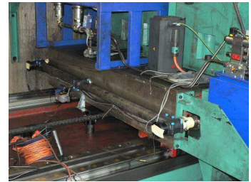
Pic. 2 – Unloaded composite frame with laser cage
