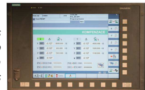
User environment on Siemens 840D control system used to control compensation in an individual axis
