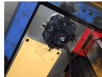
Pic. 4 – Laser measurement of shift and rotation of the RAM end
