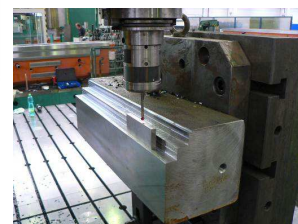
Measuring with a touch probe on a WRD150 machine
