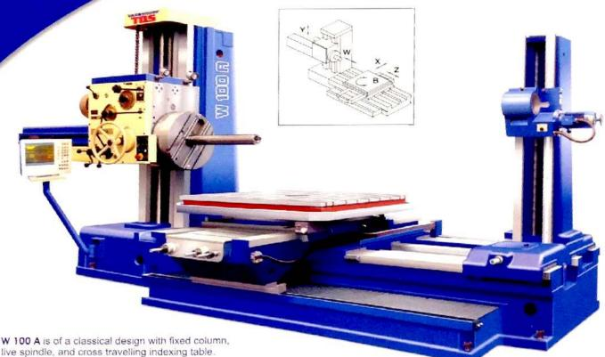
W 100 A is of a classical design with fixed column, live spindle, and cross travelling indexing table. Versatility of this machine is enhanced by its headstock having an integrated facing head. The machine design also allows the utilization of long boring bars armed with boring heads and supported by bar rest. For its outstanding performance W 100 A has become the most widespread product of TOS VARNSDORF a. s. As many as 5,100 machines of this model have been delivered worldwide since 1963.
