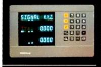
POSITIP 855 as a sophisticated DRO offers, apart of displaying position at four axes with the least increment of 0,001 mm, a lot of other useful features. These are graphic display, dialog windows, automatic offset calculations and calculator for computing of cutting conditions.
