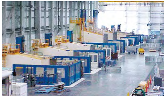
Boeing, Decatur, Alabama, USA N.8 Vertical turning milling lathes, model (AS 65 TM)
