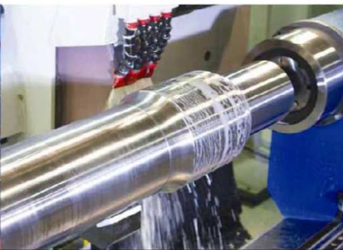
grinding of the shaft
