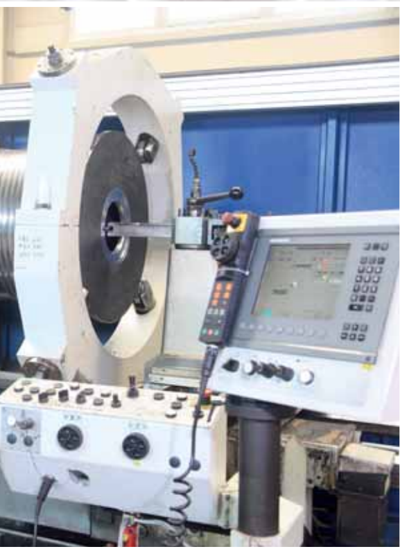
Turning of Cable Drum
