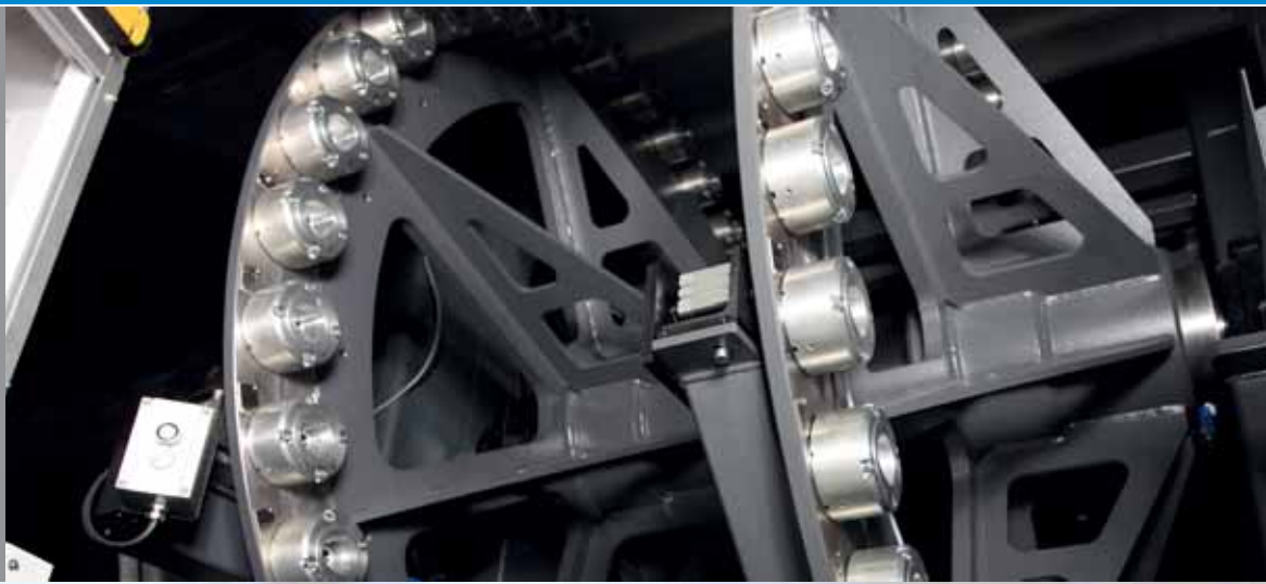
Magazine Capacity up to 120Tools
